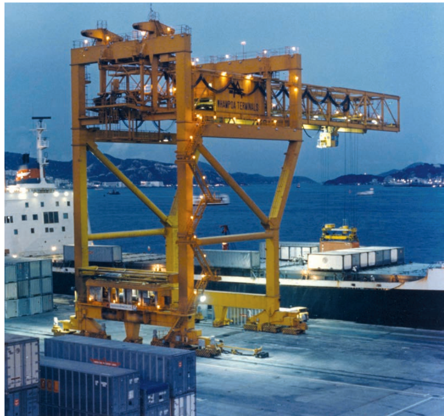
The spreaders of early quay cranes had to be positioned manually over the containers
