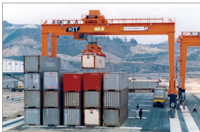
1-over-4 RTGCs would be used in the 1980s
