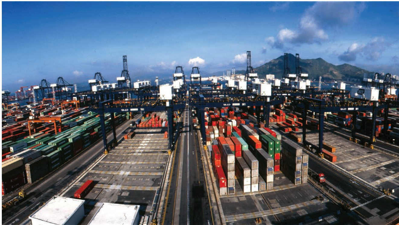
RMGCs can stack containers six high along 12 rows
