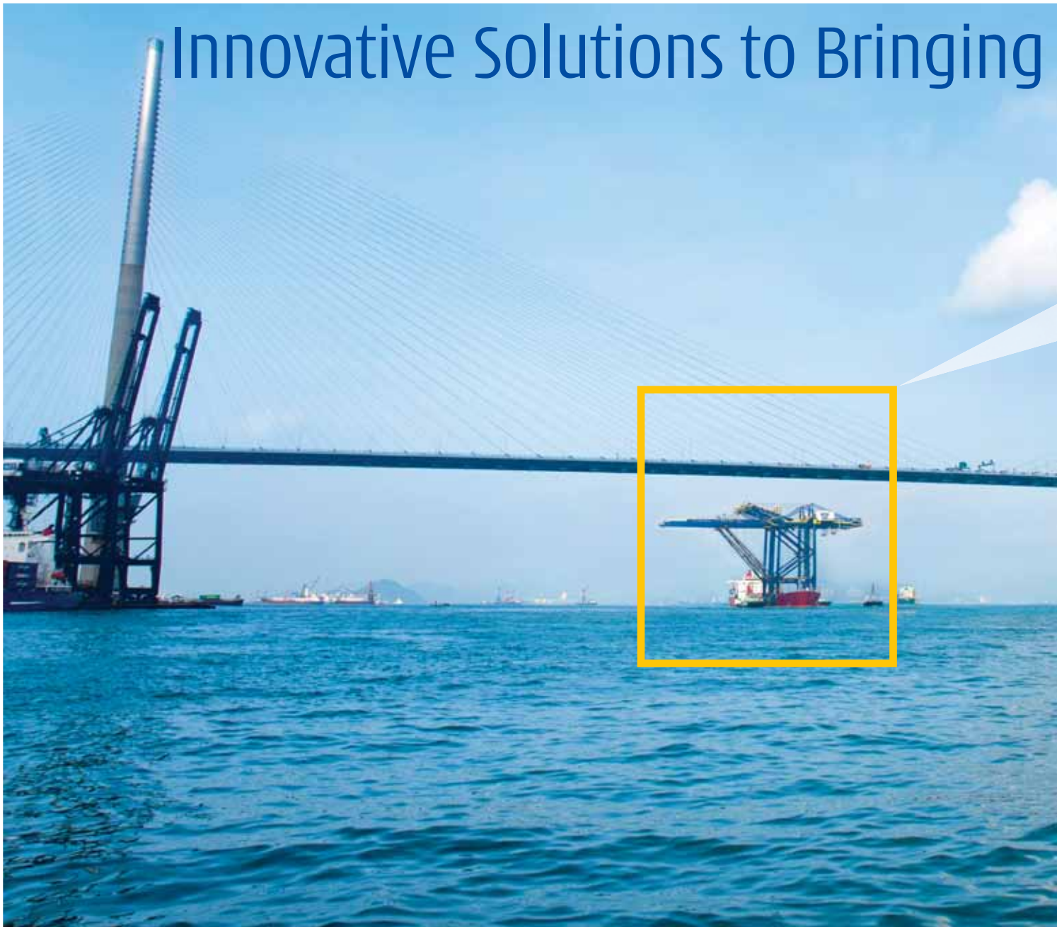
Two new quay cranes with their A-frames lowered pass underneath Stonecutters Bridge at Kwai Tsing port
